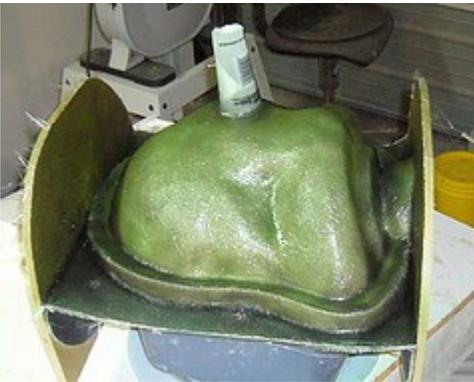
After the first two layers have cured, add additional layers as needed. In this **case**, I added 3 more layers of 1.5 oz mat to get a 1/8" lay up. 1/8" is strong enough for a **mold** of this size. Large (heavier molds may require additional thickness).
