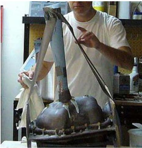
Do you see the tall funnel I have? This is because height = pressure. Fill the cone (keep it slender. A fat cone wastes RTV) with RTV and as it fills, it will bleed out the holes that you drilled in the **case**. Once they bleed out a little, plug the hole with a ball of clay. Add enough RTV so that the entire **case** fills and there is an inch or two left in the funnel.
