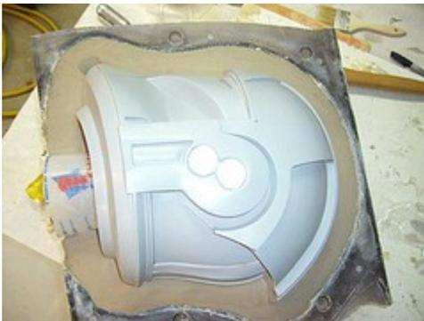
Once you have a nice clean edge tooled into the clay, add some keys so the rubber registers back into the same place each time. I use acrylic hemispheres, but you can also poke depressions into the clay with a drill bit. It works the same.
