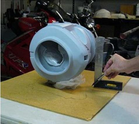
When you have made enough points to connect the dots you will have an outline of the model that can be cut out with a saber saw.
