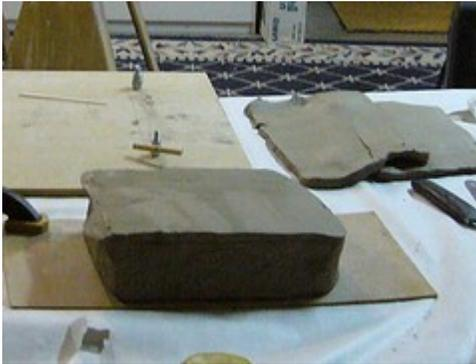
Here is the model covered with 1/2" of clay + a gasket edge. That is a lip that helps hold the rubber in the shell. The edges slope at 2-3 degrees to lock the rubber in. It also gives the rubber more of a mating surface when the **mold** is assembled.
