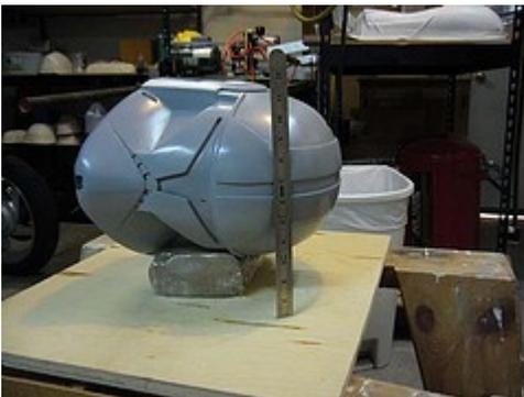
In order to get a good parting line from the Masonite, I use a square and a pen to mark the outline of the model. Simply go around the model with the square and mark the outer most points of the model.
